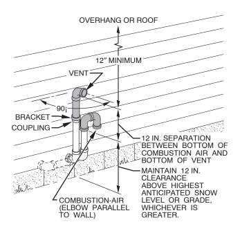
Fig. 43—Sidewall Termination of Less than 12 in.
